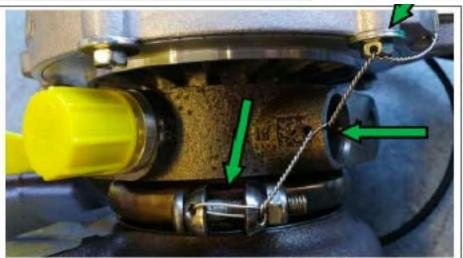
Example how to route wire through housing and exhaust (base part + mounting bolt)
