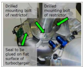
two restrictor mounting bolts. Seal tag number shall be visible from upwards
